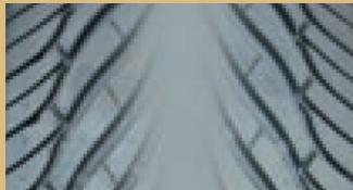
**Tracking Problems** – Excessive wear around the inside or outside edges of your front tyres could mean your front suspension has been knocked out of line through hitting a deep pothole or banging against a kerb. Ask your tyre dealer to check your car's tracking; if it is out of alignment, getting it fixed will reduce the abnormal tyre wear and make your car feel much better to drive.
